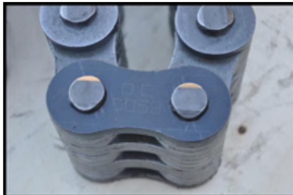
**Batch Serial number on selected side plates on all Dongbo Chain. Every batch QA tested and recorded for material, heat treatment and workmanship**
